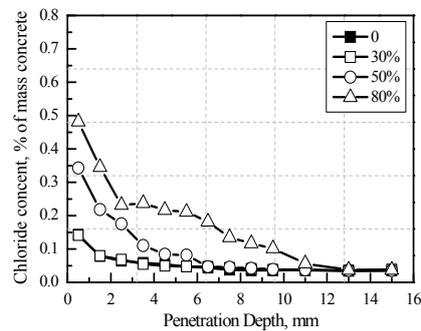
Figure 8: Chloride profiles as determined in damaged HPFRCC after self-healing.
