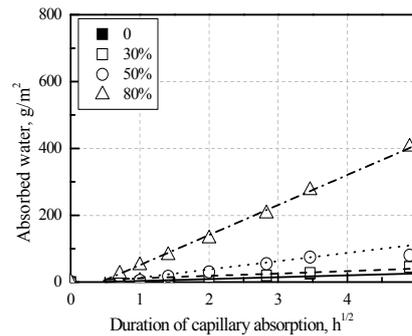
Figure 3: Influence of an applied tensile stress on capillary absorption after unloading
