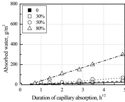
Figure 4: Capillary absorption of pre-damaged HPFRCC after unloading and self-healing
