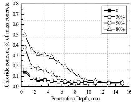
Figure 7: Chloride profiles of pre-loaded HPFRCC after direct contact with 5% NaCl for 28 days
