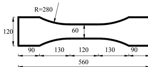
Figure 1: Shape and dimensions of the dumbbell specimens with a thickness of 30 mm
