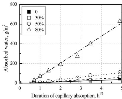
Figure 2: Influence of an applied tensile stress on capillary absorption of HPFRCC
