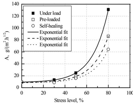
Figure 5: Coefficient of capillary absorption as function of the applied stress level
