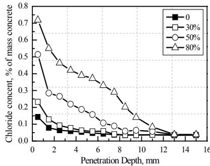
Figure 6: Influence of imposed stress on chloride penetration into HPFRCC under tensile stress after direct contact with 5% NaCl for 28 days
